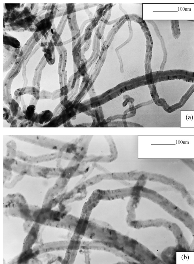
Fig. 3. TEM image of different CNTs (a) pristinine CNTs and (b) CNTs after Fenton/UV treatment.
